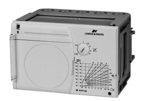
Heating control system for use in smaller plants. Control of boiler temperature through direct burner control, pump control, weather-compensated setpoint (with or without room temperature influence), or room temperature compensation.
