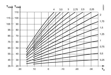
Outside temperature [°C] Flow temperature with a base point at 20 °C Flow temperature with a base point at 35 °C
